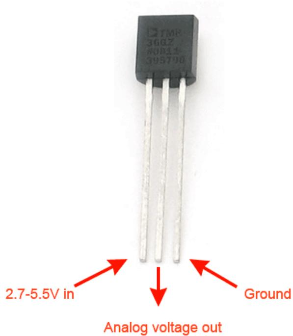
A Temperature sensor like TM36 use a solid-state technique to determine the temperature.
